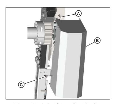
Figure 6–6: Drive Shroud Installation
