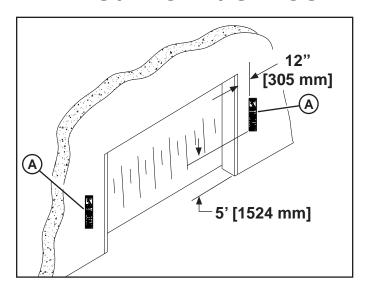
Figure 6-5: Label(s) on Back Side of Door
