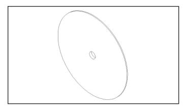
Figure 1–4: Backing Plate - 1/8" [3 mm] x 6" [152 mm] Ø
