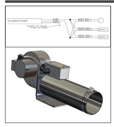
Figure 1–9: Thermal Air Seal Blower Installation
